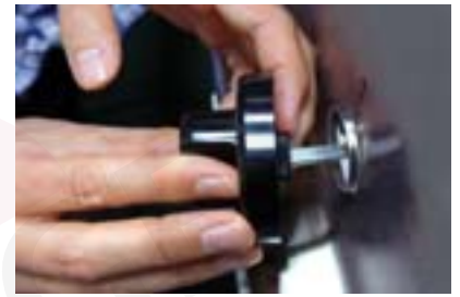
3 Push the knob on the adapter. (Note the zero position)
