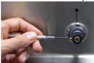
2 Screw the adapter to the round spindle ...
